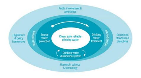
Figure 3: Multiple-Barrier Approach to Drinking Water Protection
