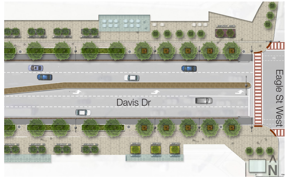
Plan of a signalized intersection along the Davis Urban segment of Davis Drive West
