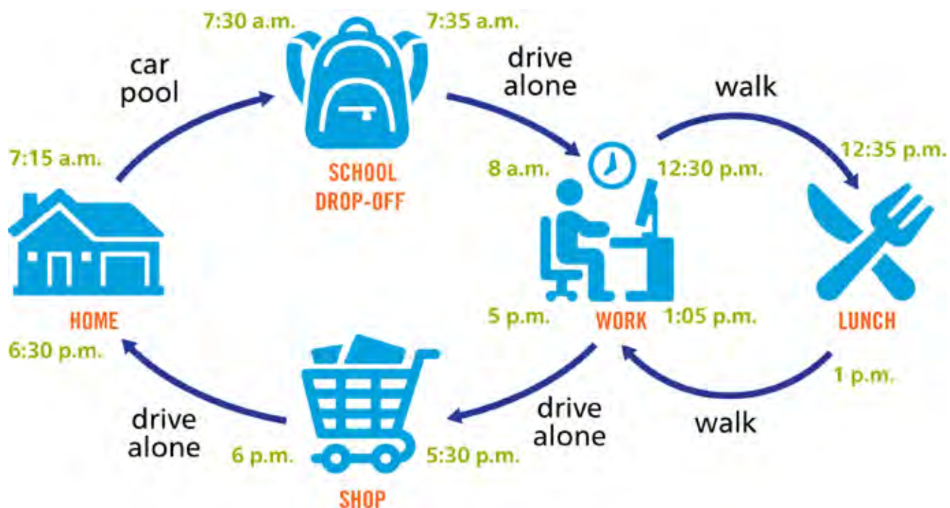
▲ FIGURE 12: York Region's activity-based model estimates all trips over a 24-hour period to help forecast the impacts of growth on the transit and roads networks.
